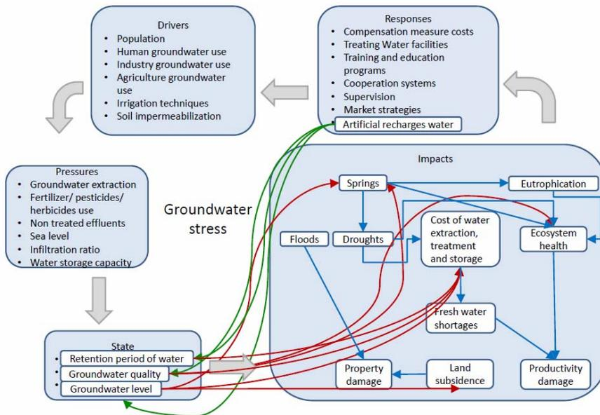
Fig. 3 – Managed aquifer recharge role in the DPSIR model.
