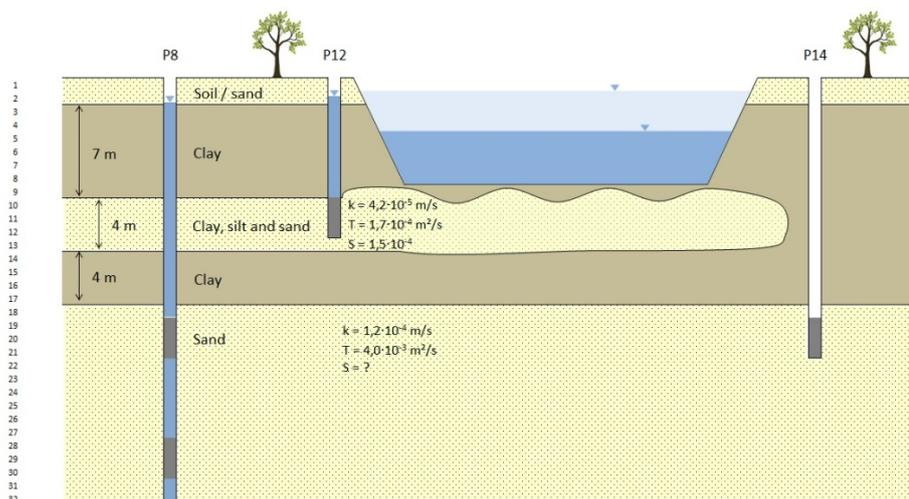
Fig. 6 - Hydrogeological Conceptual Model for Copparo
