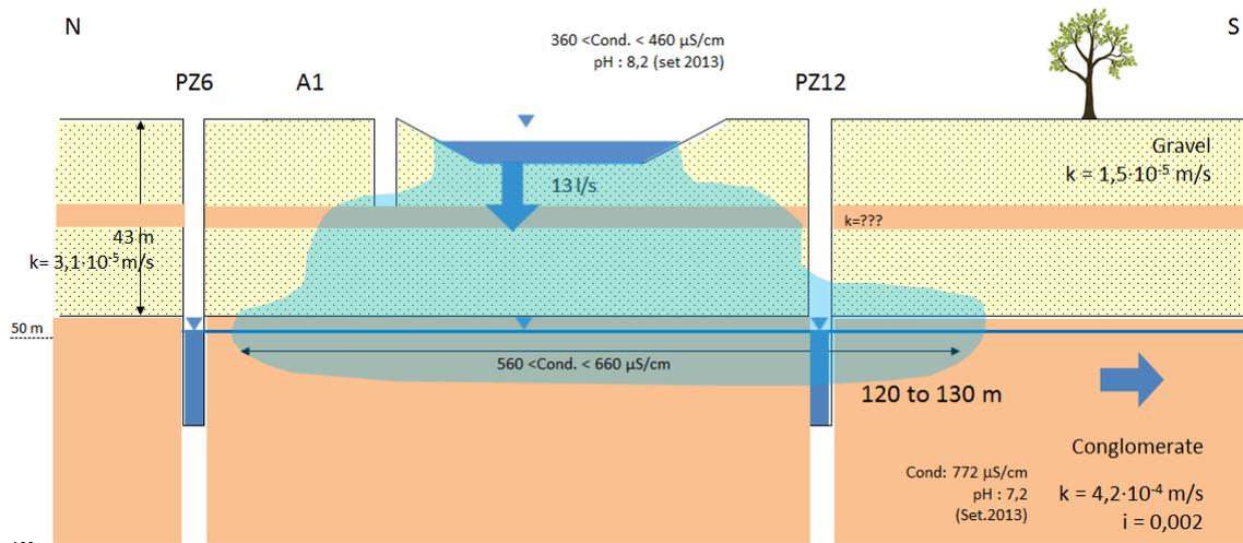
Fig. 5 – Hydrogeological Conceptual Model in Mereto
