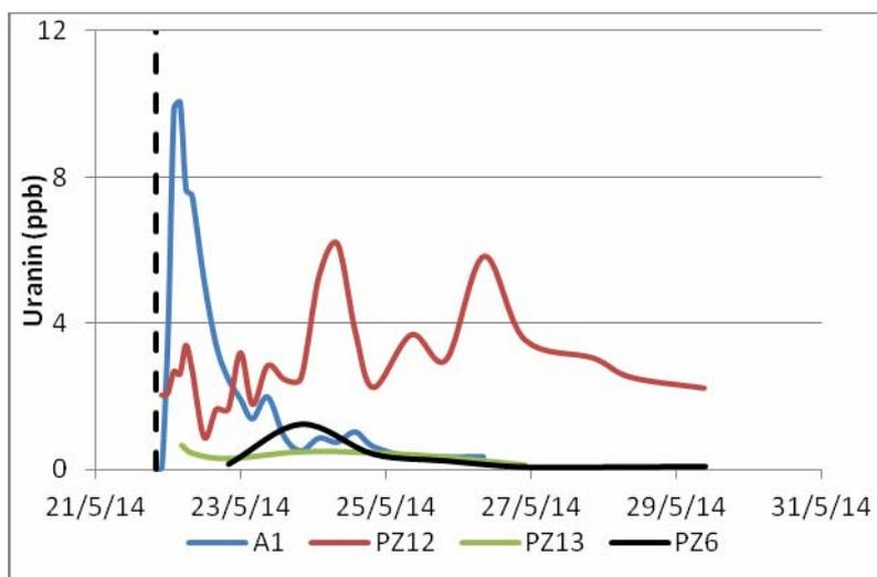
Fig. 1 – Tracer test results in the different monitoring wells (tracer begun at 20h on the 21<sup>st</sup> May, with a injection of 10 g of tracer)
