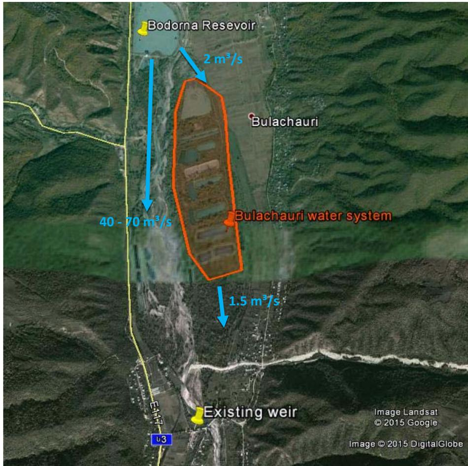
The main issue is to evaluate the possible effect on the Bulachauri water system due to the lowering of water level in the Aragvni river, according to environmental flow (5 m<sup>3</sup>/s), as this condition may increase the hydraulic gradient and the rate of water loss in the Bulachauri water system actually estimated 0.5 m<sup>3</sup>/s. In a very simplified way the possible effect of water diversion is shown in the following figure.
